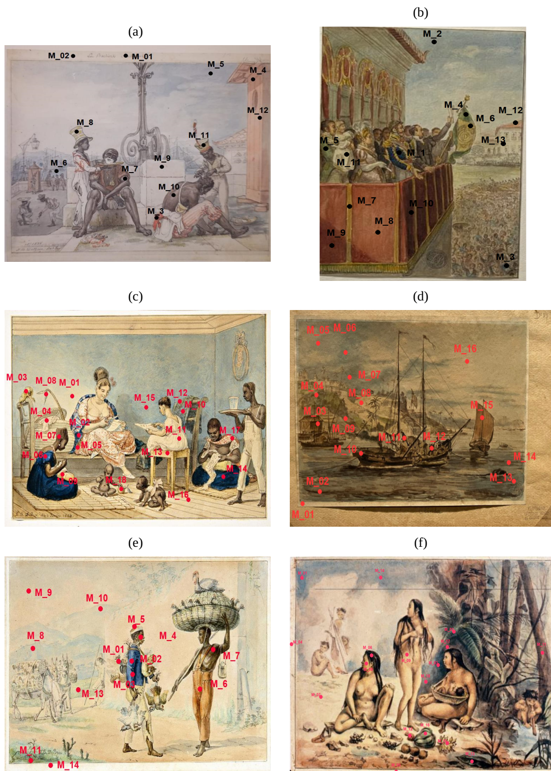
Figure 4 - Description of the images showing the points analyzed by FTIR in the watercolor prints. Prints considered authentic: (a) 3CM, (c) 1CM, and (e) 4CM; and prints considered suspicious: (b) 8CM, (d) 6CM, and (f) 7CM.
