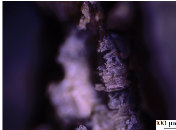
Figure 7 - Fractured section of a specimen after a tensile test. Magnification 5X.
