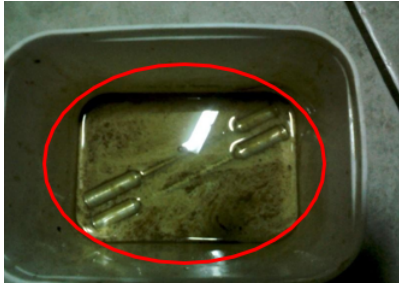
Figure 11 - Test specimens immersed in cutting fluid.
