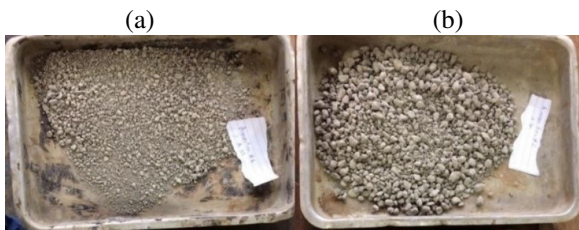
Figure 4 – Particle size obtained after crushing the concrete blocks: (a) size fine and (b) size coarse.
