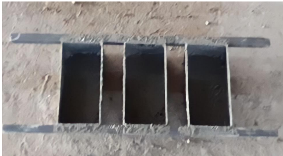
Figure 5 – The cast used in the production of the pavers.
