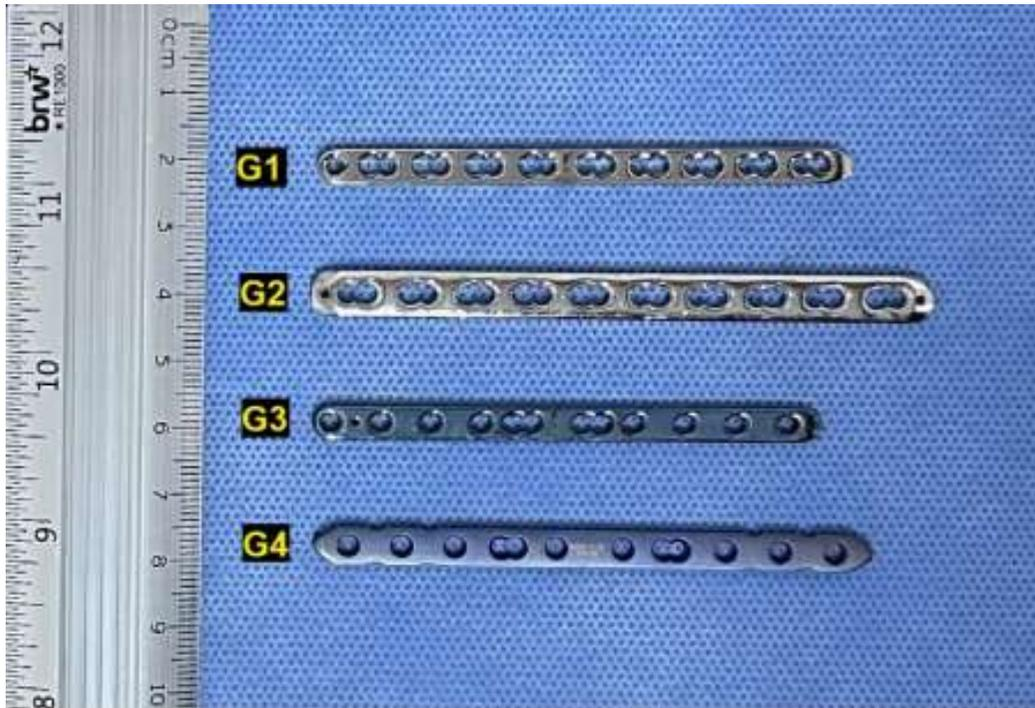
**Figure 1.** Locking compression plates in F138 stainless steel (G1 and G2) and F67 titanium (G3 and G4), respectively.
