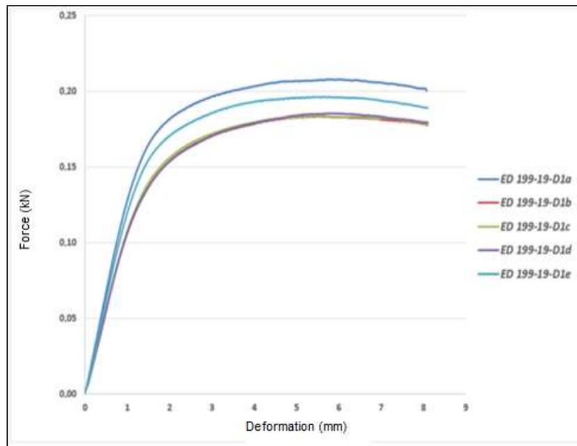
**Figure 7.** Force-deformation curves obtained in the static axial compression test for the LCPs of G4, with the maximum bending load in N being obtained (a); 0.2% yield strength in N (b); bending strength in N/m (c); bending stiffness in N/mm (d), and structural bending stiffness in N/m<sup>2</sup> (e). The curves represent the progressive action of the force applied to the loading rollers and the consequent elastic and plastic deformation caused to the tested plates.
