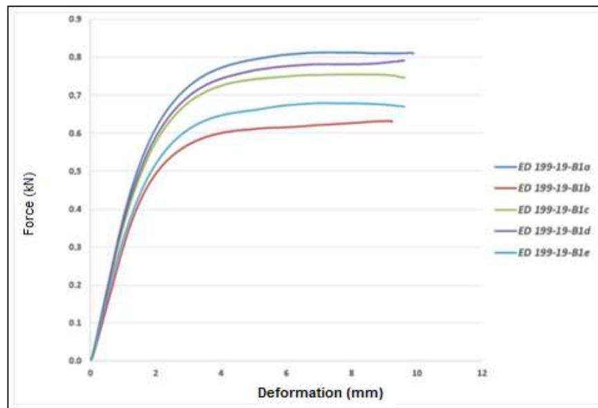
**Figure 5.** Force-deformation curves obtained in the static axial compression test for the LCPs of G2, with the maximum bending load in N being obtained (a); 0.2% yield strength in N (b); bending strength in N/m (c); bending stiffness in N/mm (d), and structural bending stiffness in N/m<sup>2</sup> (e). The curves represent the progressive action of the force applied to the loading rollers and the consequent elastic and plastic deformation caused to the tested plates.
