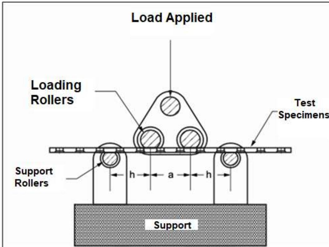
**Figure 3.** Schematic drawing of the front view of the bending device of the plate to be tested, where “h” represents the loading span and “a” the central span.
