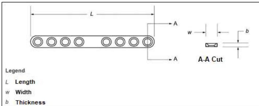
**Figure 2.** Designation of bone plate dimensions used in this study.
