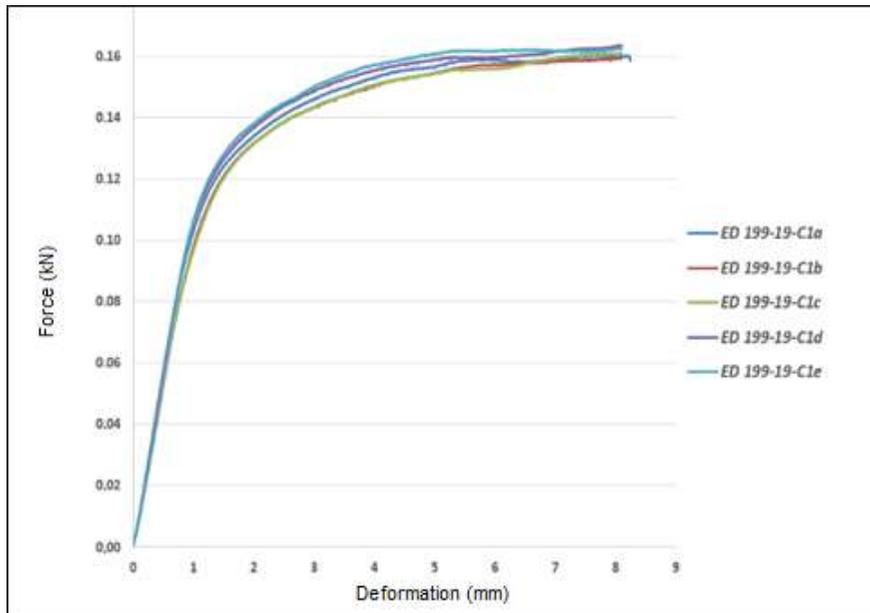
**Figure 6.** Force-deformation curves obtained in the static axial compression test for the LCPs of G3, with the maximum bending load in N being obtained (a); 0.2% yield strength in N (b); bending strength in N/m (c); bending stiffness in N/mm (d), and structural bending stiffness in N/m<sup>2</sup> (e). The curves represent the progressive action of the force applied to the loading rollers and the consequent elastic and plastic deformation caused to the tested plates.
