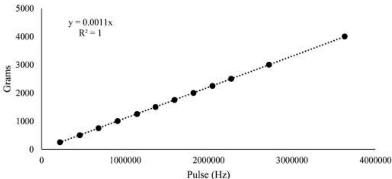
Figure 2. Scale calibration curve.
