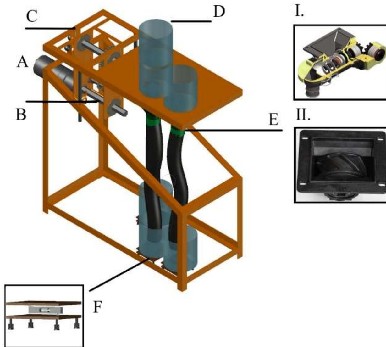
**Figure 1.** Diagonal projection of the electronic and automated static bench. Electrical control (A), transmission set (B) and articulation (C), reservoirs (D), dosing mechanisms (E) simple helical (I) and fluted (II) and the data acquisition system (F).
