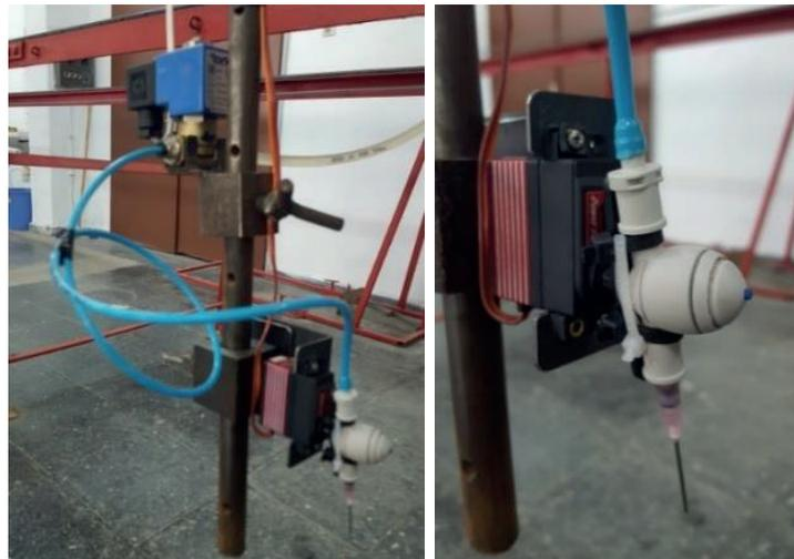
**Figure 4.** Servomotor coupled needle nozzle.
