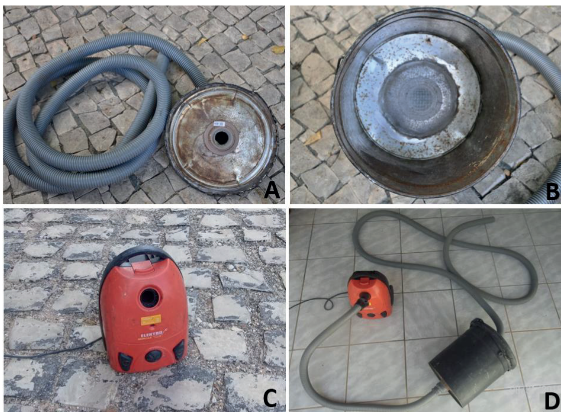
Figure 1. Swarm Suction Device. Suction device prepared by the SOS Abelhas Project Team to capture wild swarms of Africanized honeybees ( Apis mellifera L.) in the city of Mossoró, RN, Brazil.
