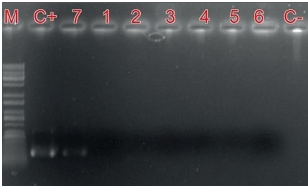
Figure 1. Nested-PCR results, shown on a 2% agarose for Leptospira spp. from free-living capybara ( Hydrochaeris hydrochaeris ) serum samples from a university campus in the city of Araras in São Paulo, Brazil, 2013-2014. 1 molecular marker (100 bp) (Invitrogen®, Brazil); 2 C+, positive control; 7 sample with DNA amplification (331 pb); 1, 2, 3, 4, 5 and 6 tested samples; C-, negative control.
