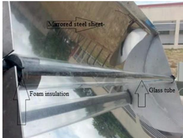
Figure 5. Mirrored steel sheet, glass tube and foam insulation.
