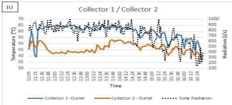
**Figure 12.** Results of experiment 3: (a) Collector 1 data; (b) Collector 2 data; (c) Comparison of collector outlet temperatures.
