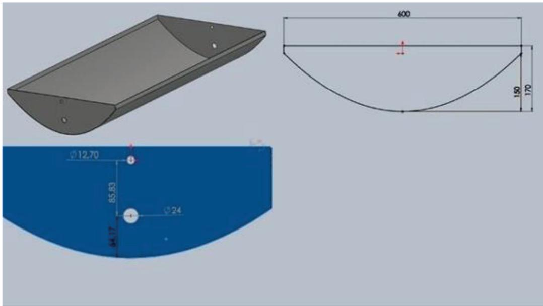
**Figure 3.** Parabolic reflector.
