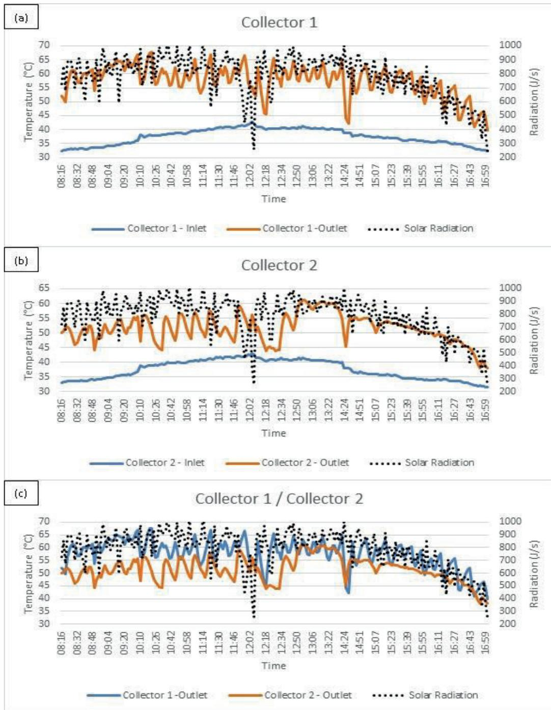
**Figure 16.** Results of experiment 5: (a) Collector 1 data; (b) Collector 2 data; (c) Comparison of collector outlet temperatures.
