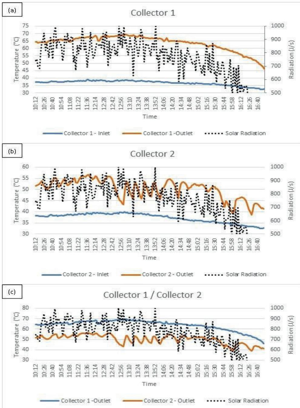
**Figure 14.** Results of experiment 4: (a) Collector 1 data; (b) Collector 2 data; (c) Comparison of collector outlet temperatures.
