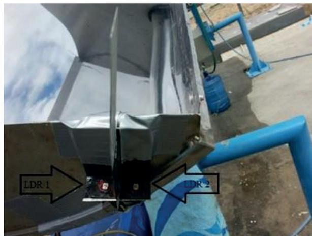
Figure 6. Disposition of LDRs for tracking.
