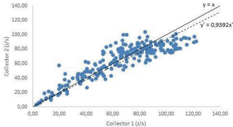
Figure 11. Comparison of absorbed energy results in experiment 2.
