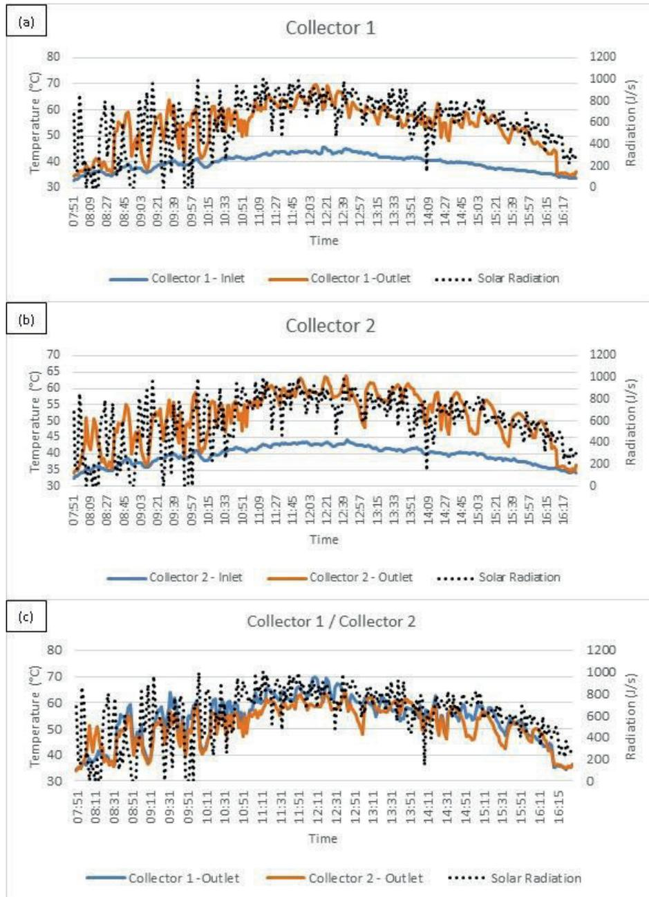
**Figure 8.** Results of experiment 1: (a) Collector 1 data; (b) Collector 2 data; (c) Comparison of collector outlet temperatures.
