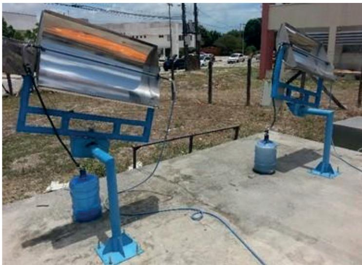
**Figure 4.** Parabolic Trough Collectors installed.
