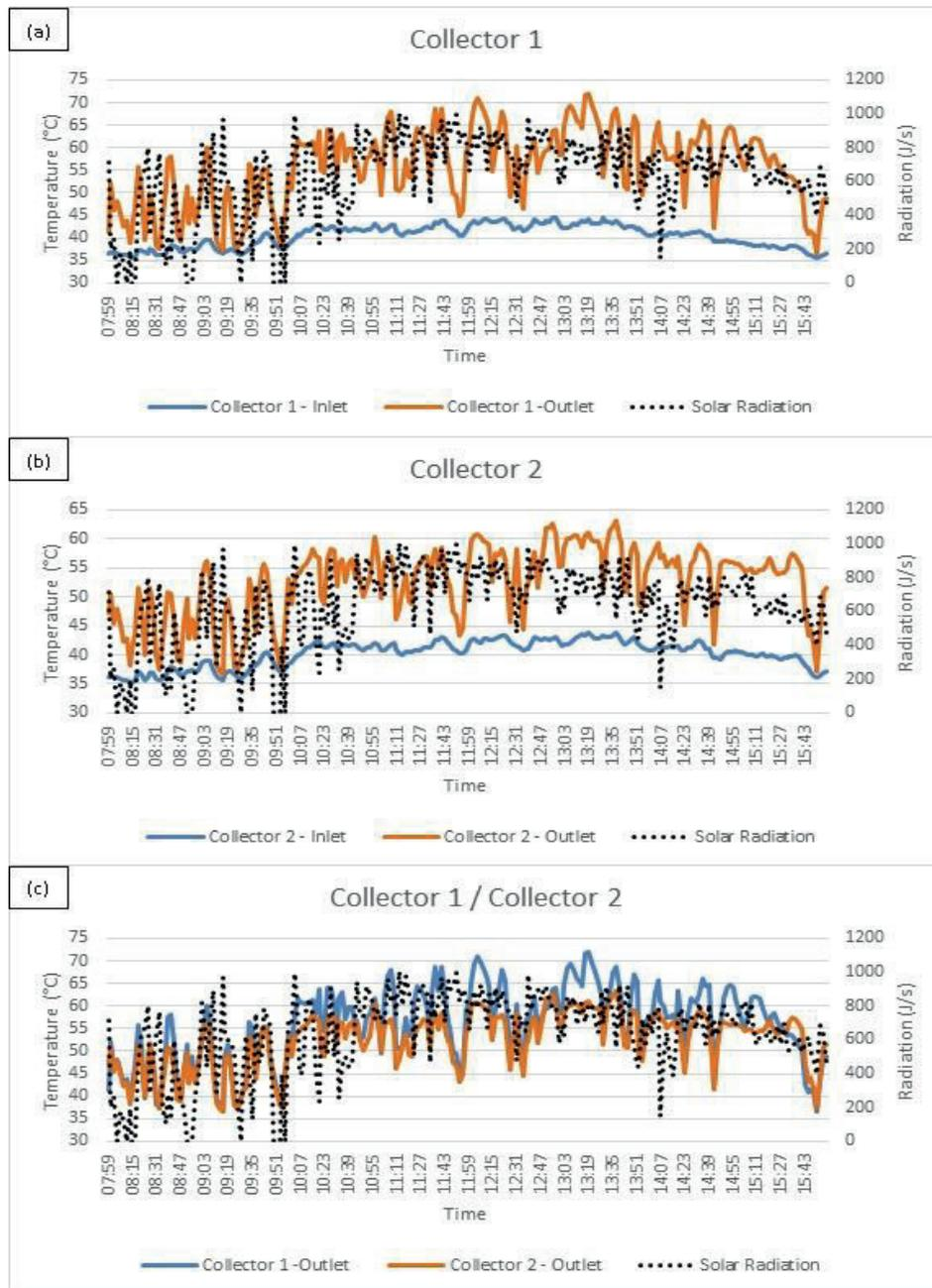
**Figure 10.** Results of experiment 2: (a) Collector 1 data; (b) Collector 2 data; (c) Comparison of collector outlet temperatures.
