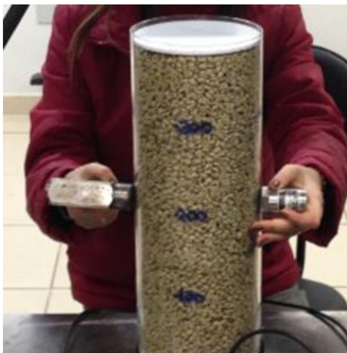
Figure 2. Stress Wave Timer coupling position in the reference silo.
