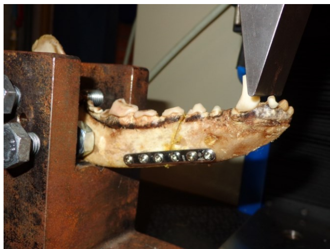
Figure 4. Dog hemimandible positioned for the biomechanical test. Note the force being applied to the incisor teeth.
