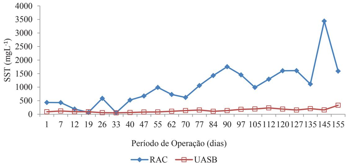
The ABR and UASB reactors presented separately mean TSS removal efficiencies of 77.5 and 75.1%, respectively, and the ABR-UASB reactor system showed a global removal of 98%.
