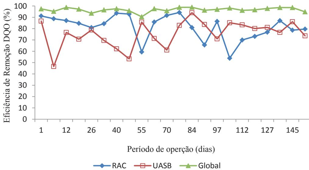
The ABR-UASB reactor system had an average removal efficiency of 96.7% for COD, with minor variations, showing high reliability and operational stability.
