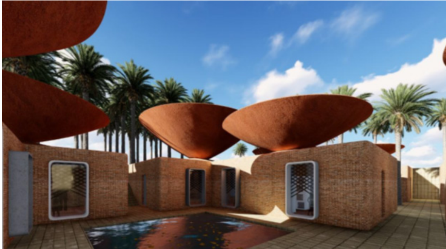
Fig. 16 - Concave Roof System Collects Rainwater. Result of the Googlestorming application
